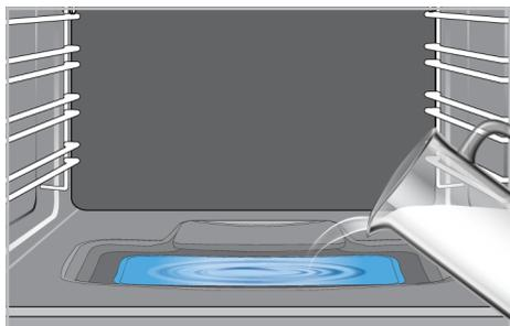
**i** Do not use distilled or filtered water. Use ready-made waters only. Do not use flammable, alcoholic or solid particulate solutions instead of water.
